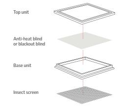
Mounting of blinds is done most conveniently during the rooflight installation process.
