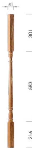
1100mm Spindle 1100 x 41 x 41mm Plain : PS02A Fluted : FS02A Roped : RS02A
