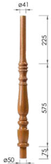
Continuous Handrail Post 800 x 91mm Plain : HP01C Fluted : FHP01C Hex : HHP01C
