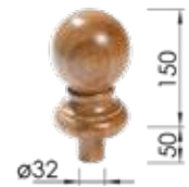
Ball Top Newel Cap 150 ex 100mm Ø32mm Dowel BT10C
