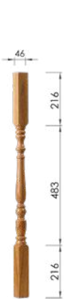
915mm Spindle 915 x 46 x 46mm Plain : PS01C Fluted : FS01C Hex : HS01C
