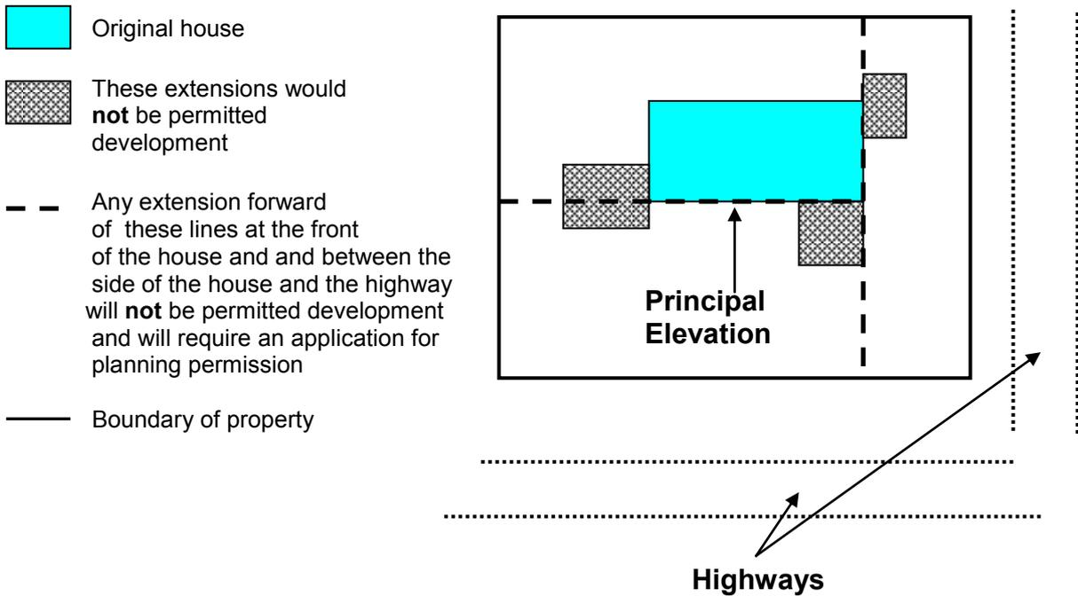
The extent to which an elevation of a house fronts a highway will depend on factors such as:
