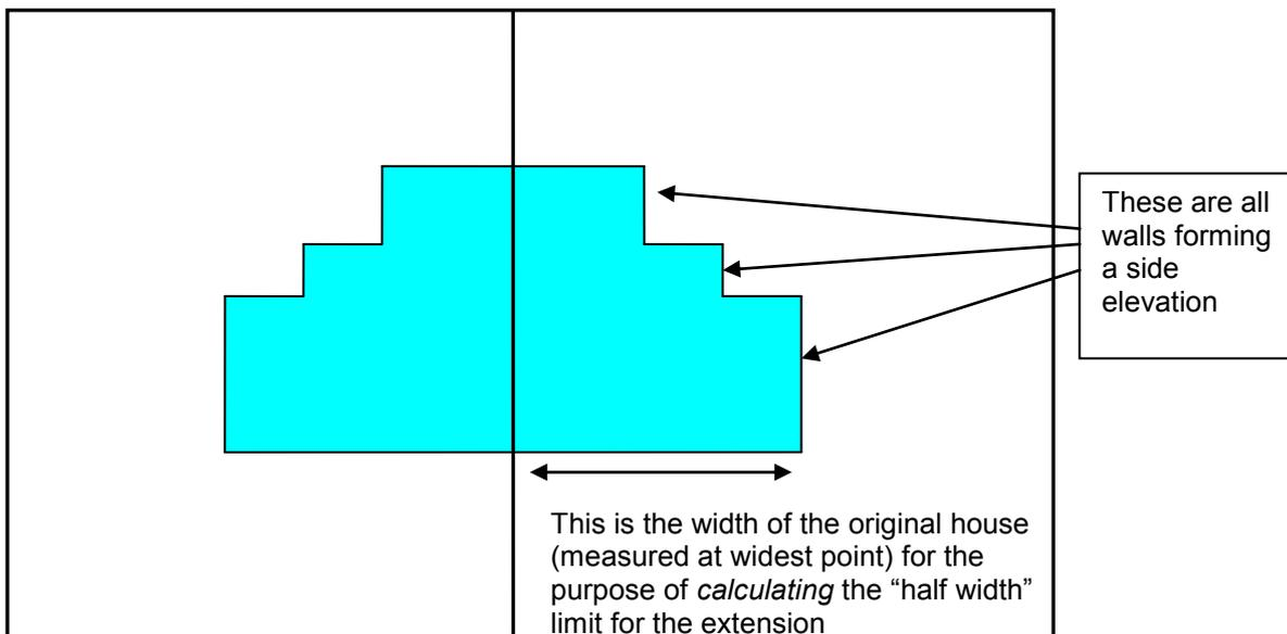
Where an extension is beyond any side wall, the restrictions in (j) will apply. Any extension can only be a single storey, must be less than 4 metres in height and can only
