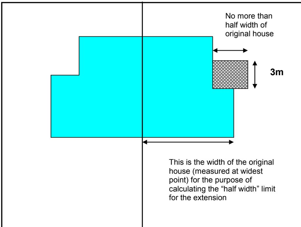
The following examples, however, would not be permitted development. In each case, the extension extends beyond a side wall and is more than half the width of the original house. An application for planning permission would therefore be required.
