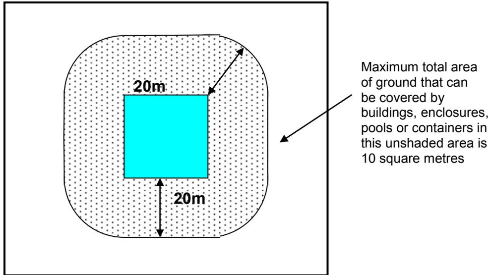
***E.3 In the case of any land within the curtilage of the dwellinghouse which is article 2(3) land, development is not permitted by Class E if any part of the building, enclosure, pool or container would be situated on land between a wall forming a side elevation of the dwellinghouse and the boundary of the curtilage of the dwellinghouse***
