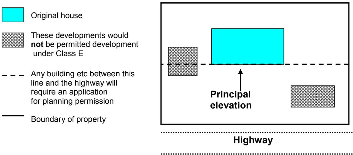
Where the principal elevation comprises more than one wall facing in the same direction, all such walls will form part of the principal elevation and the line for determining what constitutes 'extends beyond a wall' will follow these walls:
