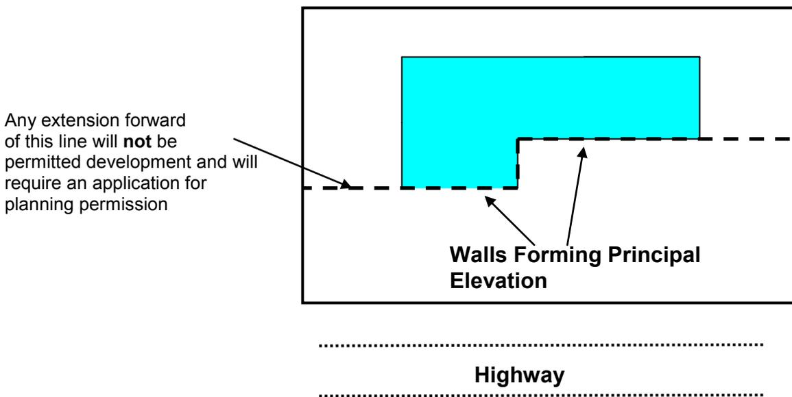
If a house sits on a corner plot where a side elevation fronts a highway, there will be an additional restriction on permitted development to the side of the house.
