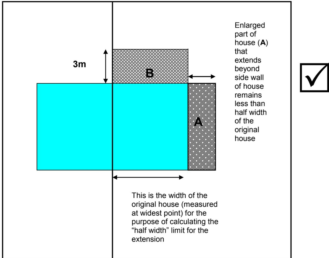
**(ja) any total enlargement (being the enlarged part together with any existing enlargement of the original dwellinghouse to which it will be joined) exceeds or would exceed the limits set out in sub-paragraphs (e) to (j);**
