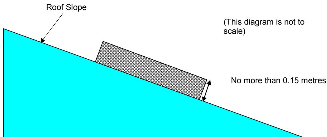
This limitation to projection from the roof plane should not be applied in cases where the roof of an extension to a house that is permitted development under Class A is joined to the roof of the original house. In such cases, the roof of the extension should not be considered under Class C as protruding from the original roof.
