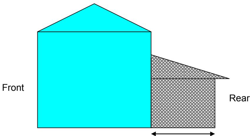
Measurement of 'extend beyond a rear wall' when the extension is directly attached to the rear wall
